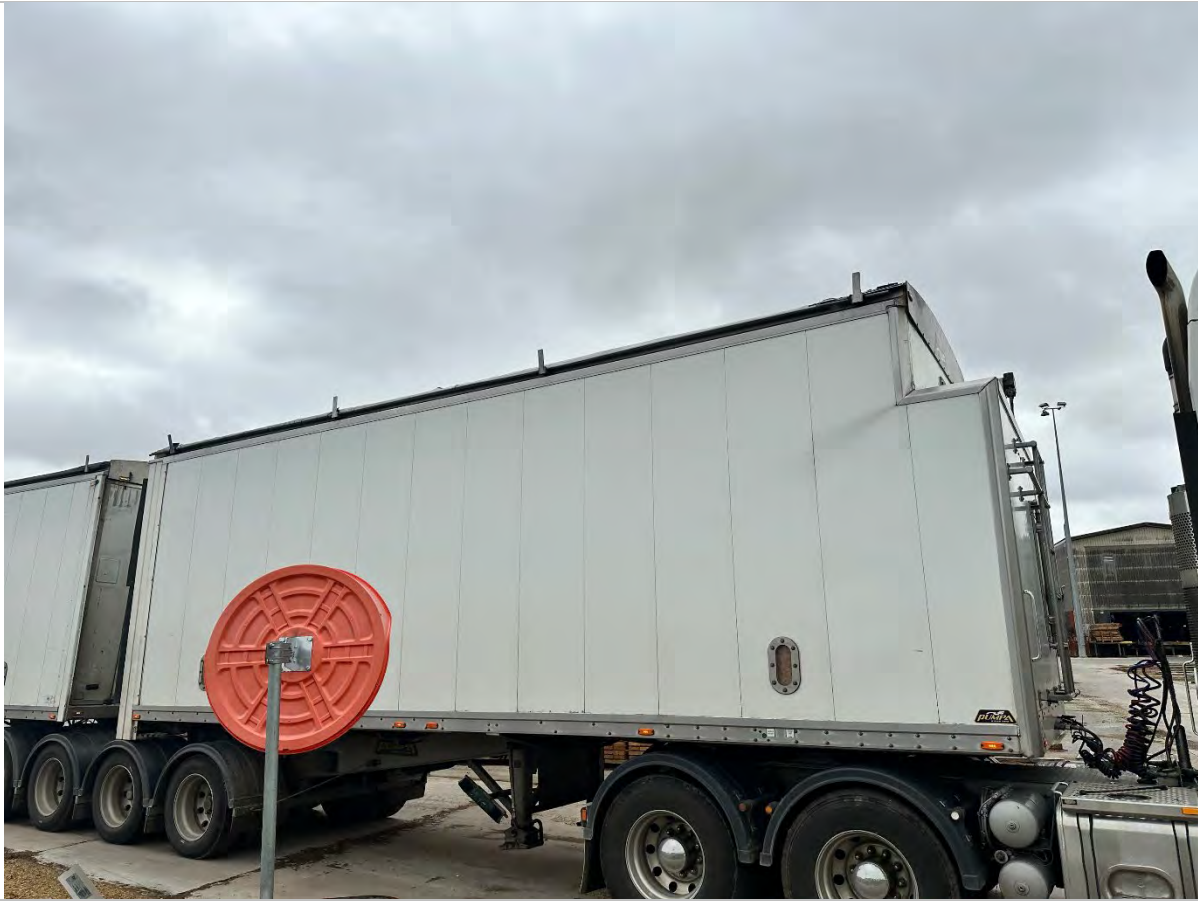
Photo 5: Dust cover on truck
